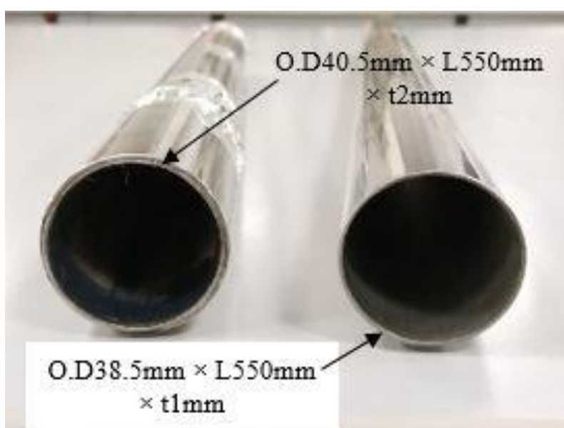
Fig. 4. 1mm and 2mm outer absorber wall thickness used for the parameter experimental setup
