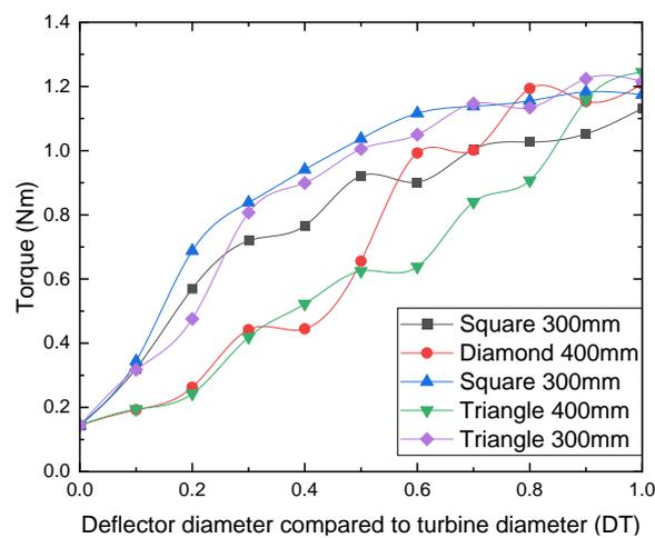
**Fig. 6.** Maximum torque produced by each deflector with optimum distance
