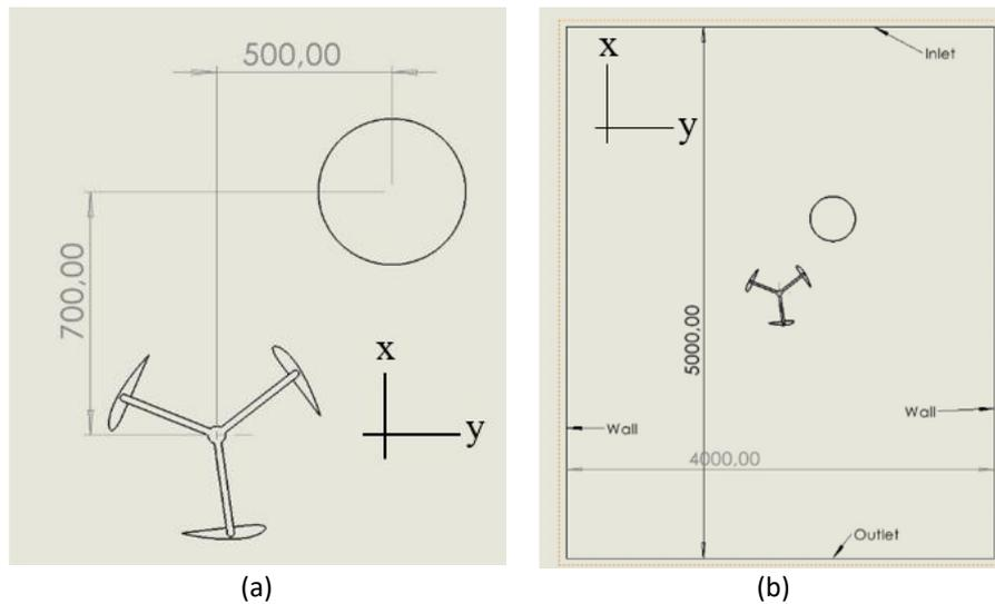
**Fig. 1.** The schematic setup for (a) Simulation setup with circle deflector, and (b) Boundary condition setup
