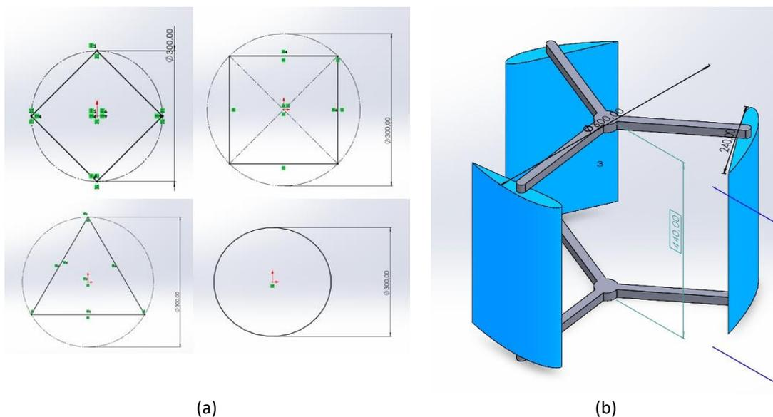
**Fig. 2.** (a) Deflectors shape and geometry, and (b) 3D model of the turbine
