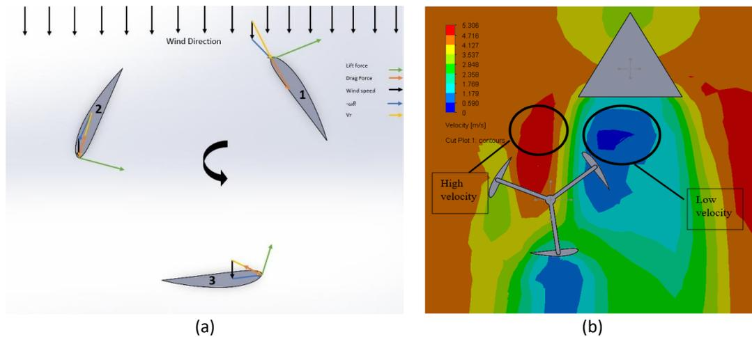
**Fig. 5.** (a) Force diagram acting on the turbine, (b) Wind flow around the turbine with triangle deflector
