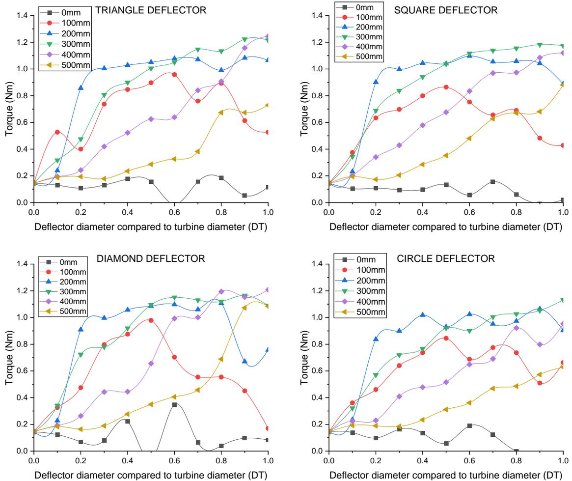
**Fig. 4.** The torque performance curves as the function of each shape of the deflector
