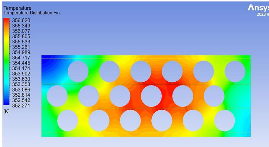
Fig. 8. Temperature distribution along fin
