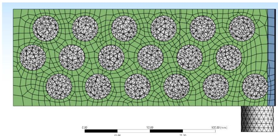
**Fig. 3.** Meshing of radiator
