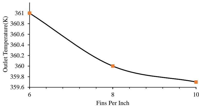
**Fig. 4.** Fins per inch vs outlet temperature
