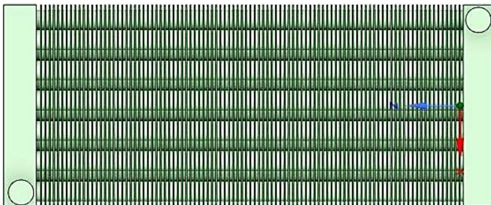
Fig. 2. Geometry of 6 FPI radiator
