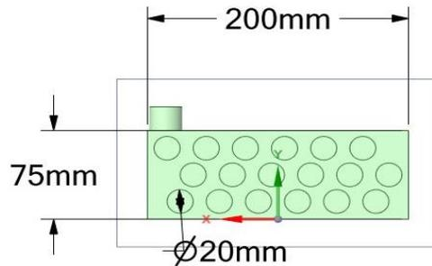
Fig. 1. Cross- section of a 6 FPI radiator
