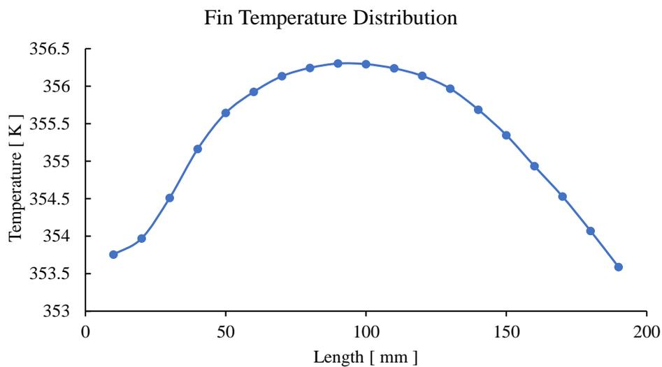
Fig. 9. Fin temperature distribution of 10 FPI radiator
