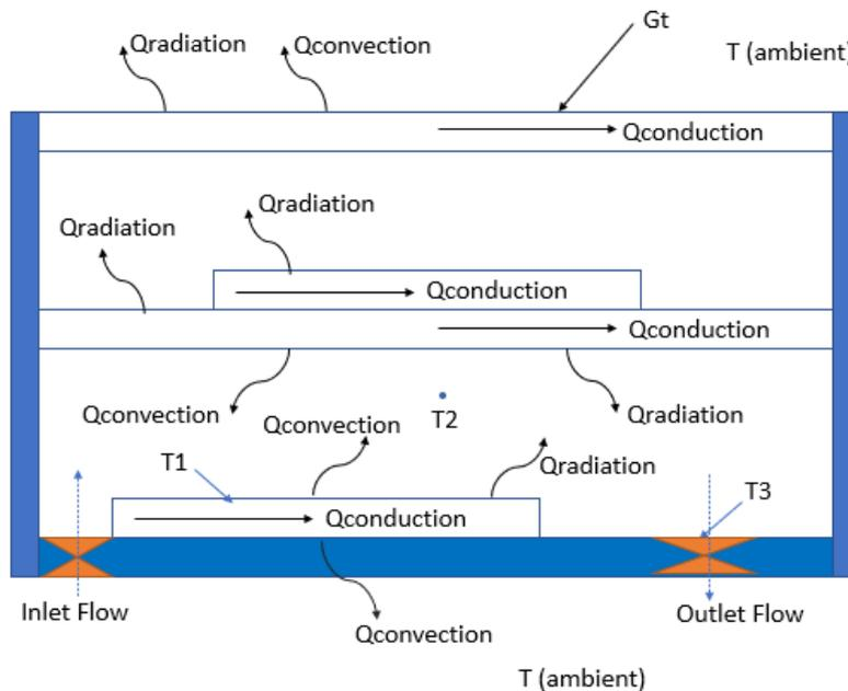
Fig. 6. Heat transfer diagram for a solar thermal collector
