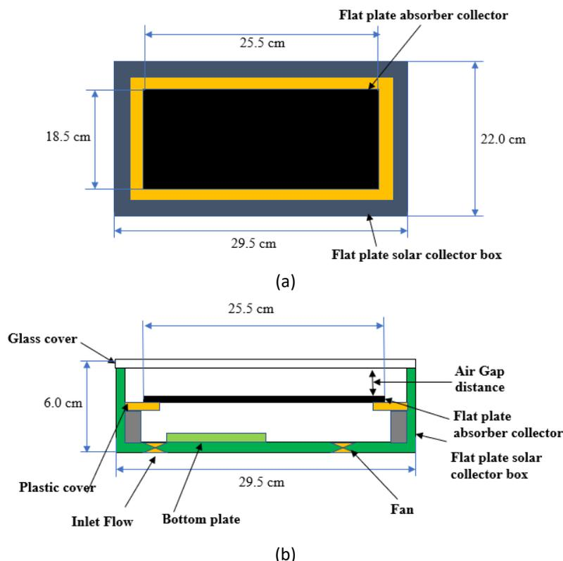
Fig. 1. (a) Top view (b) Side view of FPSC diagram
