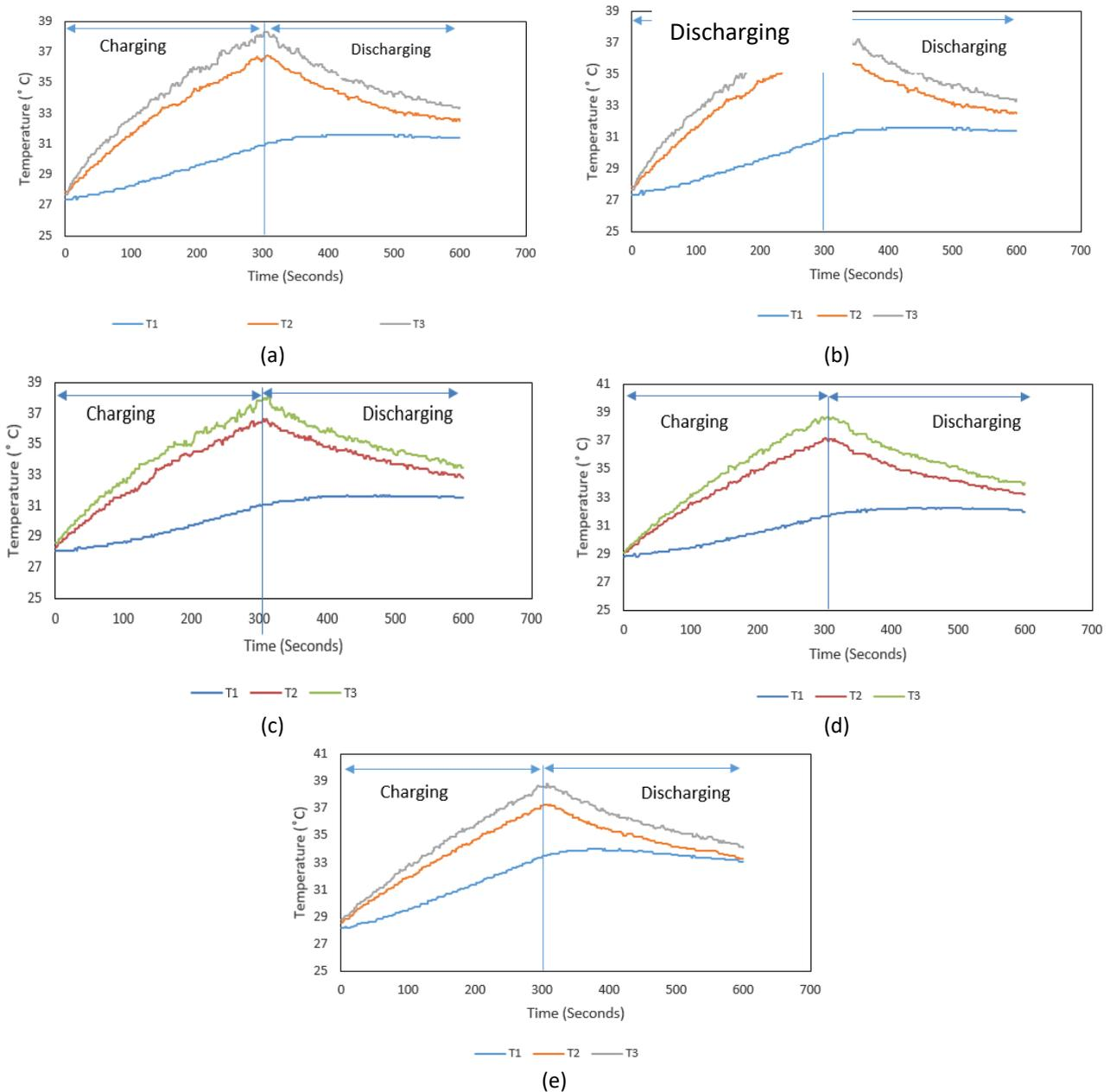
**Fig. 5.** Temperature versus time for various absorber collector configurations on (a) Case A, (b) Case B, (c) Case C, (d) Case D (e) Case E
