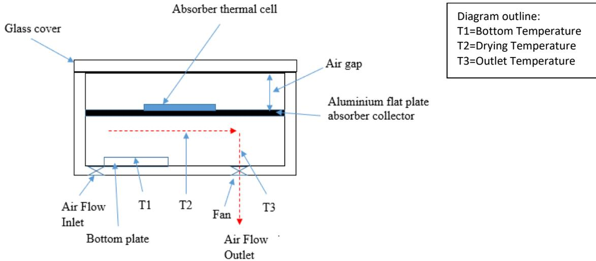
**Fig. 4. Temperature sensor location for FPBTCA**
