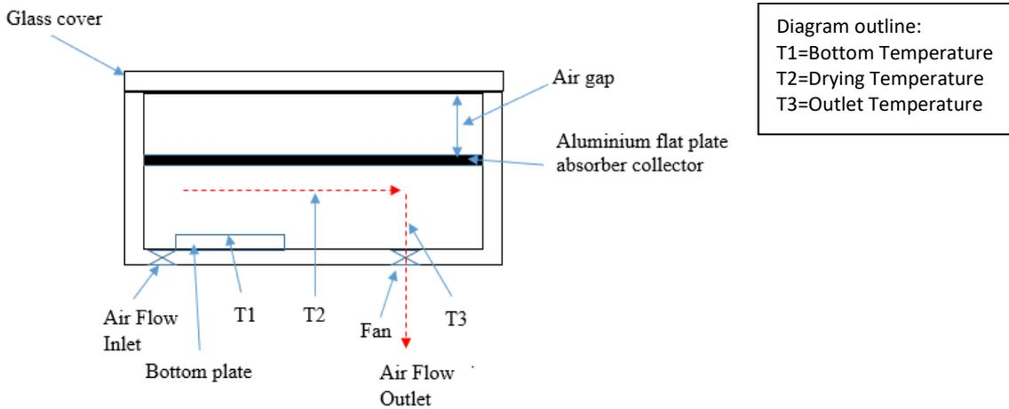
**Fig. 2. Temperature sensor location for FPSC**
