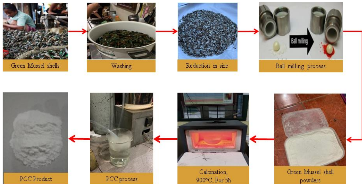
Fig. 1. The set-up experiments of green mussel shells purification with the PCC method
