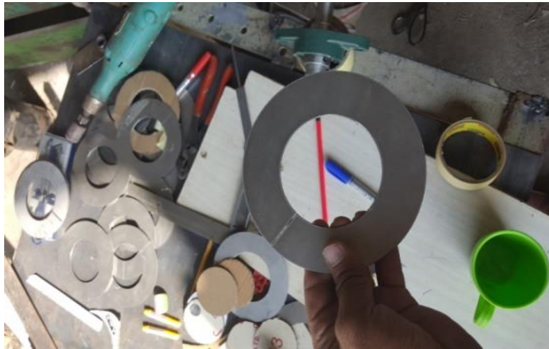
Fig. 2. The helix before welded on shaft
