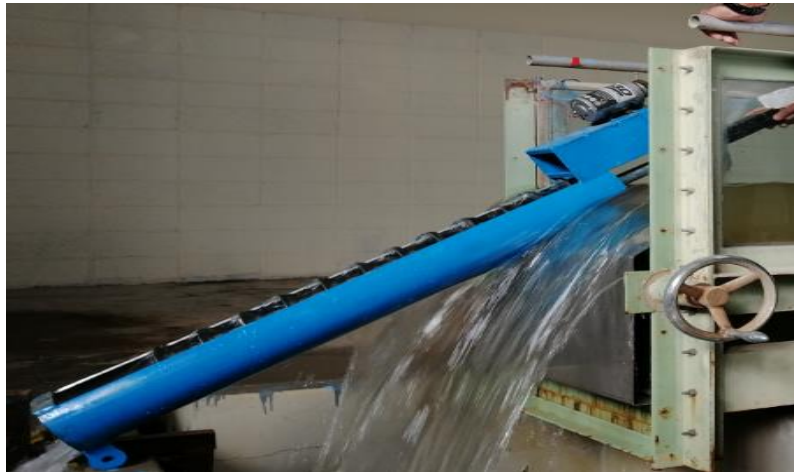
Fig. 4. Archimedes screw after completion of manufacturing
