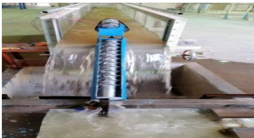
Fig. 5. Archimedes screw with hydraulic channel during operation
