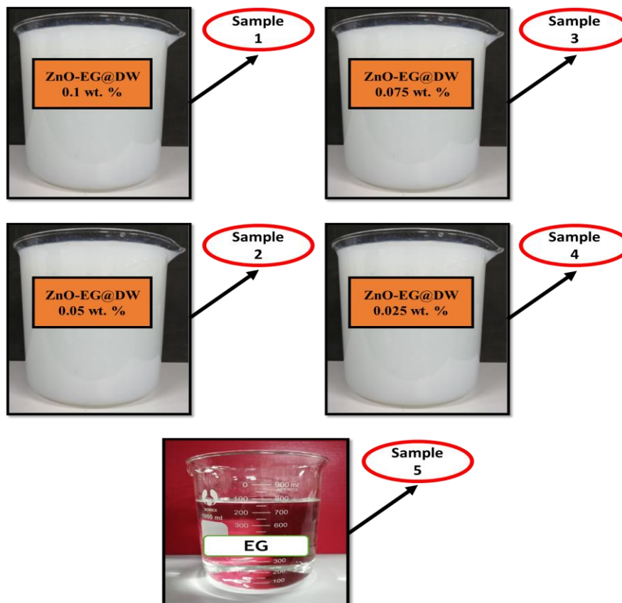
Fig. 1. (b) EG and ZnO+EG based nanofluids at varying wt.% concentrations
