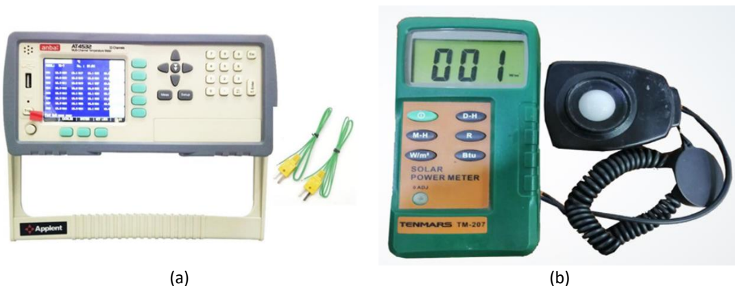
Fig. 4. Applents Digital Data Logger Thermometer (AT-4532x) 32 Channel type (a), and (b) Solar radiation measurement device (Pyranometer)
