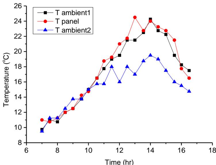
Fig. 11. Ambient and PV panels temperature for day 15 Dec
