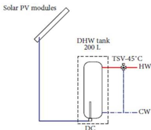
Fig. 14. Scheme of solar hot water systems (PV without MPPT) [13]
