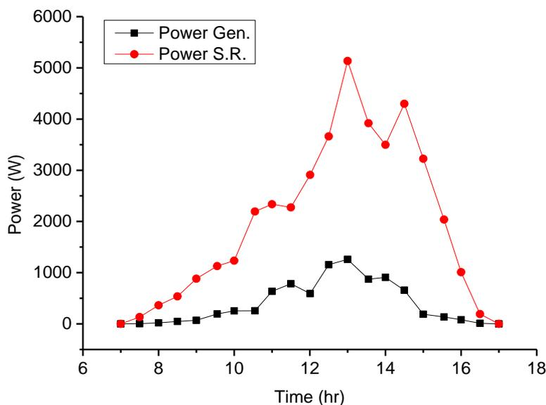
Fig. 10. Power generated and power of solar radiation with time for day 15 Dec
