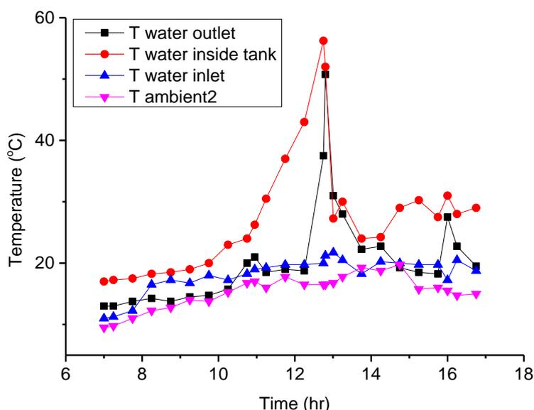
Fig. 12. Ambient temperature and water temperature for day 15 Dec
