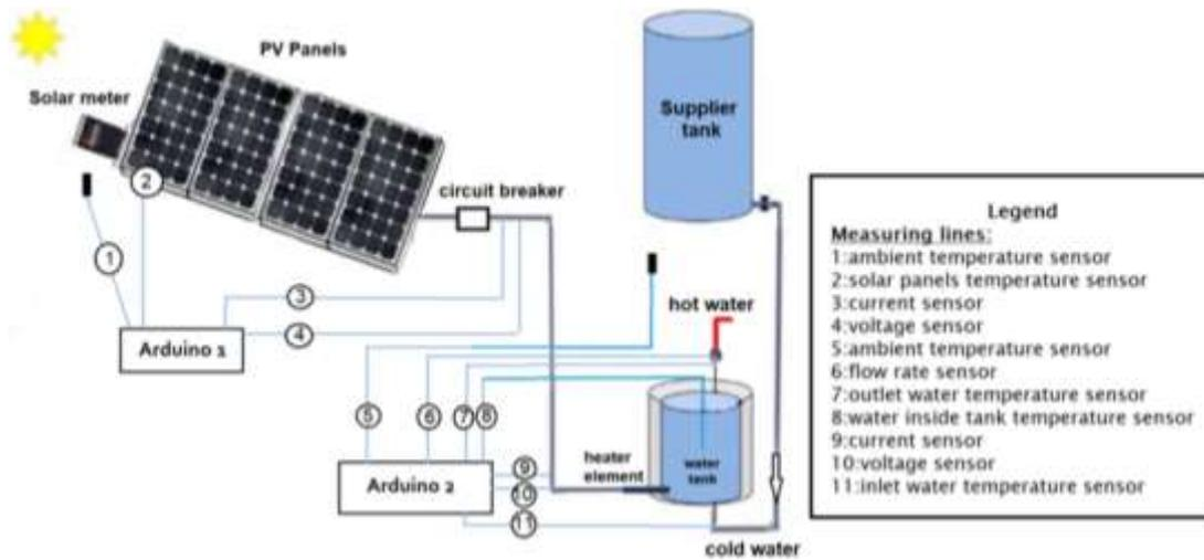
Fig. 3. A schematic diagram for the photovoltaic water heater system
