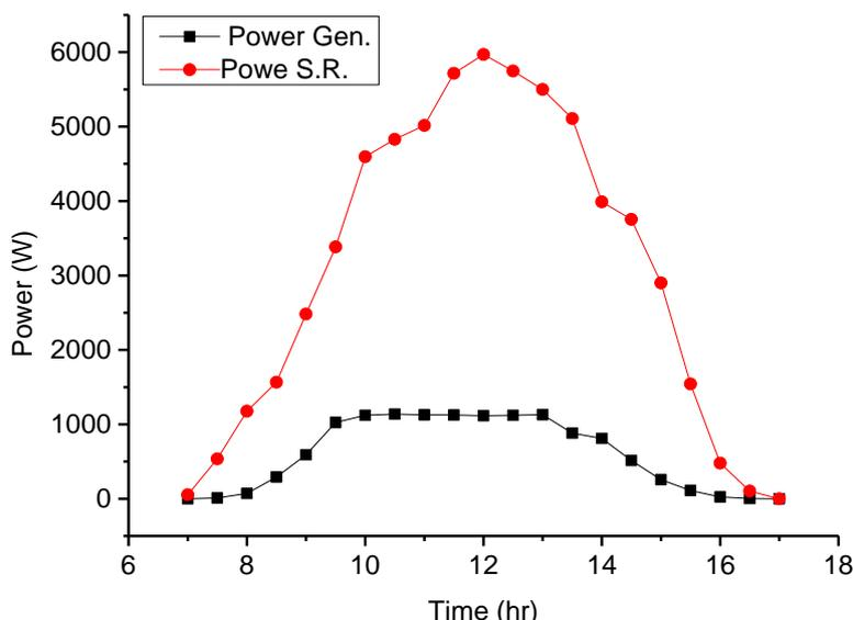
**Fig. 5.** Power generated and power of solar radiation with time for day 8 Dec
