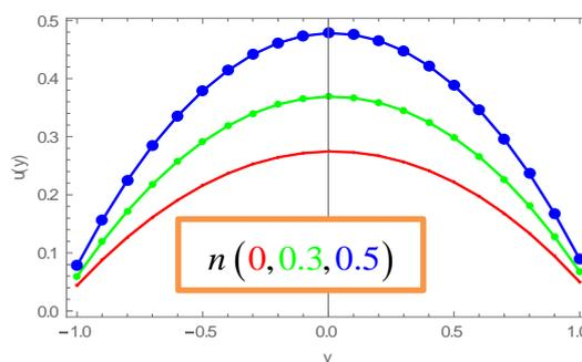
**Fig. 11.** Implications for  $n$  on velocity  $we = 0.01, \beta = 0.1, Gr = 0.5, M = 0.5, Da = 3, \phi = 0.15, Nr = 0.5, Br = 1.7, G = 0.5$
