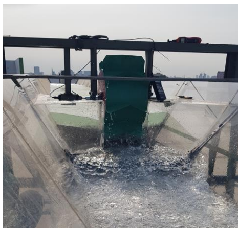
Fig. 1. Dethridge wheel experimental rig installation
