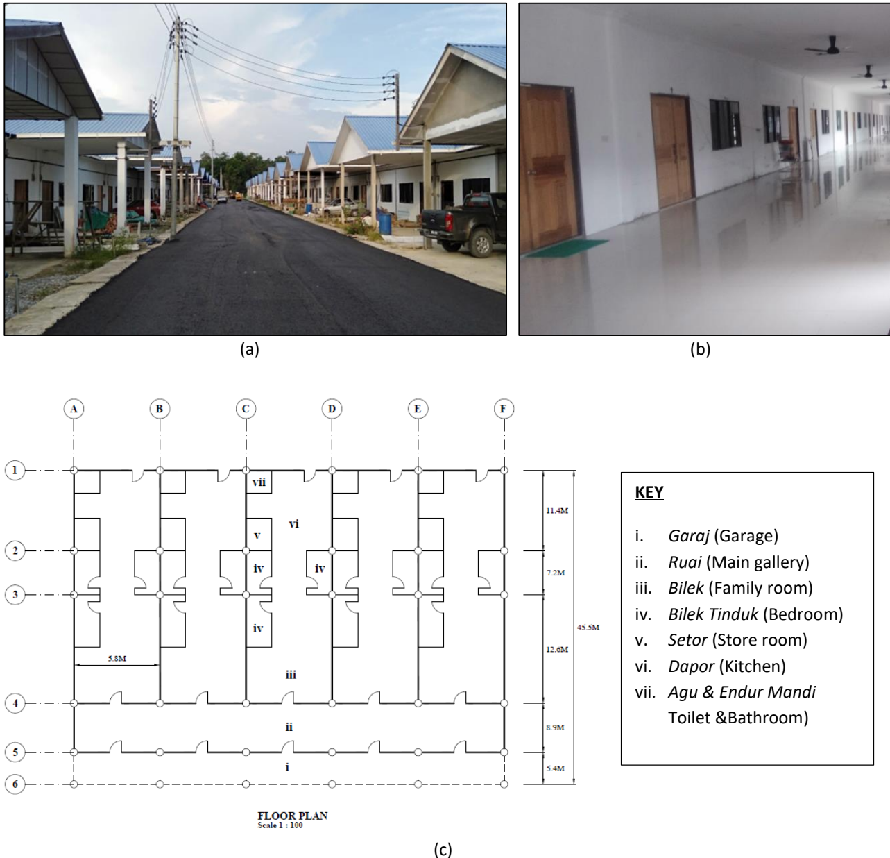
Fig. 4. (a) An example of modern longhouse, RH Tabor Ak Lasah, (b) Ruai, and (c) Floor Plan
