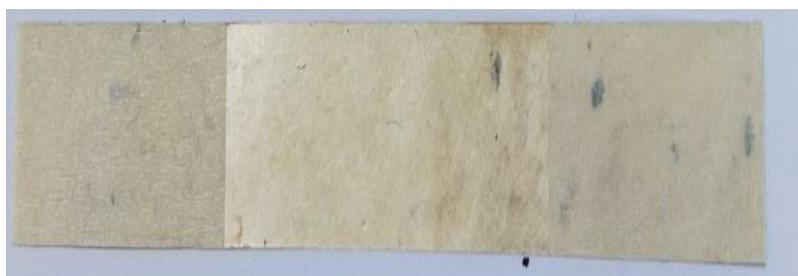
**Fig. 3.** Sample of hot-pressed kapok fiber prepared for tensile test
