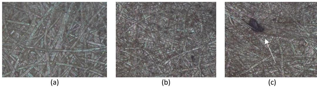
**Fig. 5.** Surface morphologies (100×) of nonwoven kapok samples hot-pressed at (a) 160°C, (b) 170°C, and (c) 180°C
