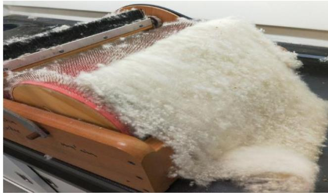
**Fig. 1.** Kapok fiber web produced using Ashford drum carder
