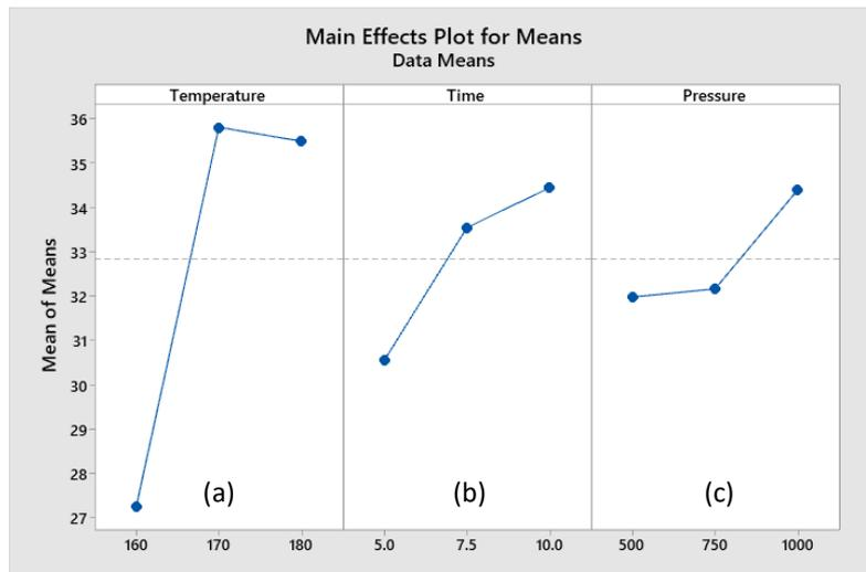
**Fig. 4.** Effect of main process parameters ((a) heating temperature, (b) heating time, (c) hydraulic pressure) on tensile strength
