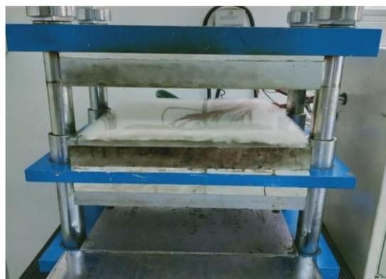
**Fig. 2.** Hydraulic hot-pressing of web kapok into nonwoven mat with higher strength
