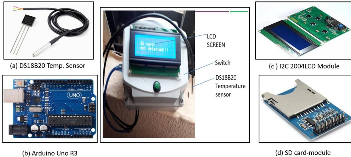
**Fig. 2.** Developed data-logger with embedded components
