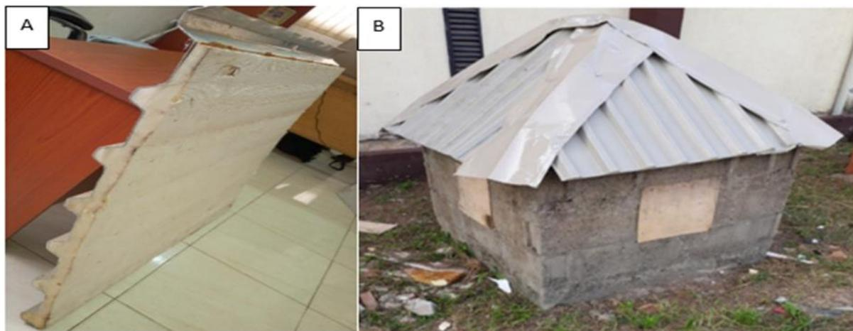
**Fig. 1.** (a) The PU embedded aluminium roofing (b) Experimental set-up of house model with aluminium polyurethane foam roofing system
