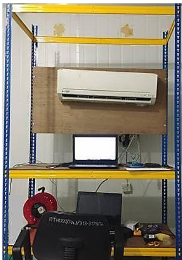
Fig. 2. Split unit air-conditioner test rig in the present work
