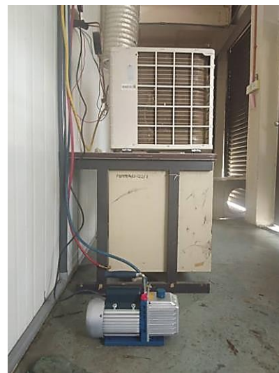
Fig. 3. Split unit air-conditioner test rig in the present work
