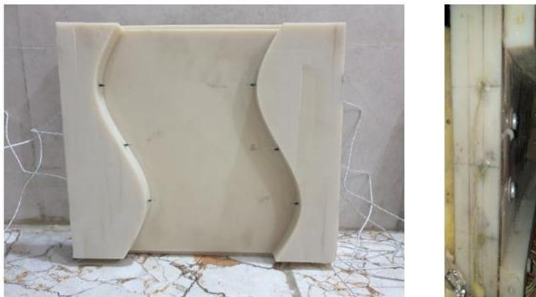
**Fig. 5.** Location of the fixed thermocouples
