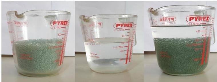
**Fig. 14.** Experimental calculation of the porosity for a glass with a diameter of 3 mm
