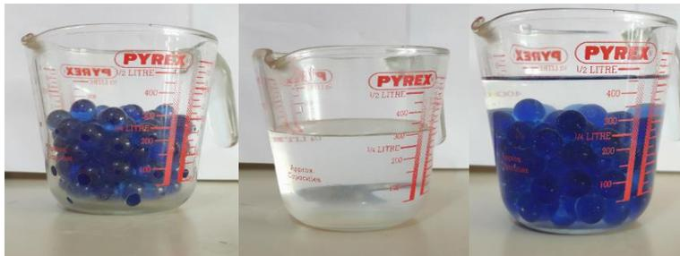
**Fig. 15.** Experimental calculation of the porosity for a glass with a diameter of 10 mm
