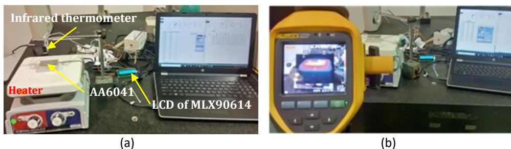
Fig. 6. (a) The temperature measurement by MLX90614 (b) The temperature measurement by Fluke Ti400
