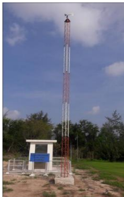
Fig. 3. The wind measuring device at the agrometeorological station [4]
