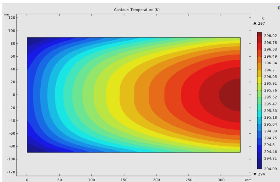
Fig. 5. Normal rectangular duct with thickness inlet dimensions 175X5 mm
