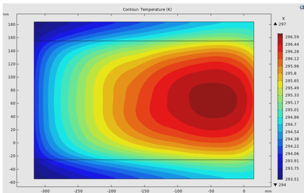
**Fig. 9.** Temperature contour for Expansion-Contraction duct with inlet 145X5 mm
