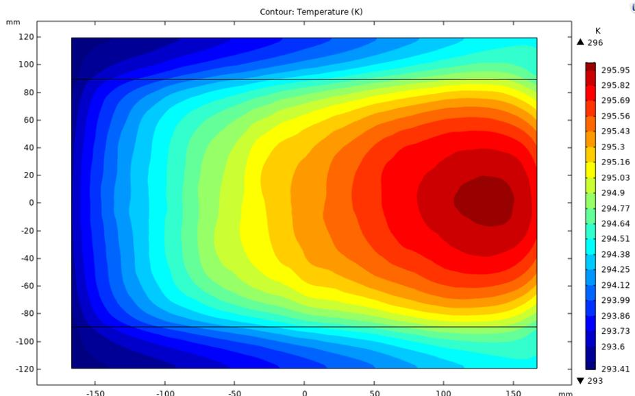
**Fig. 11.** Temperature contour for sudden expansion duct with inlet 175X5 mm
