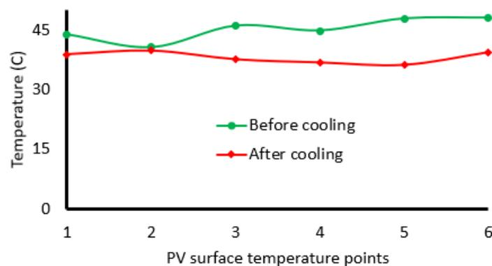
Fig. 2. PV surface point temperatures
