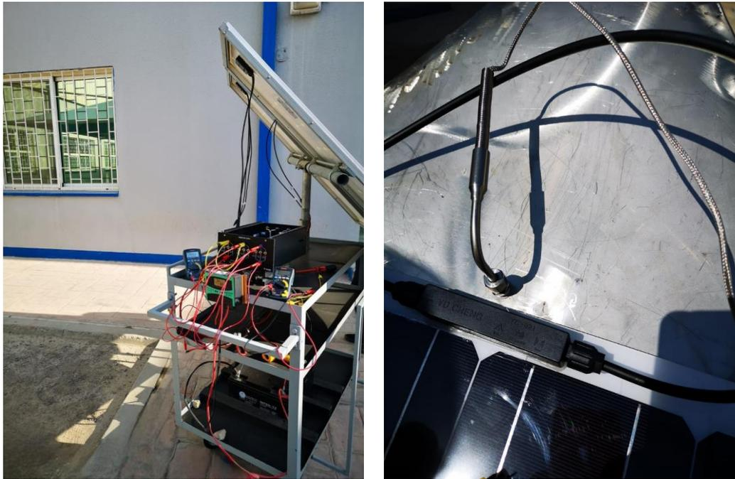
**Fig. 1.** PV system experimental with connections and thermocouple’s locations
