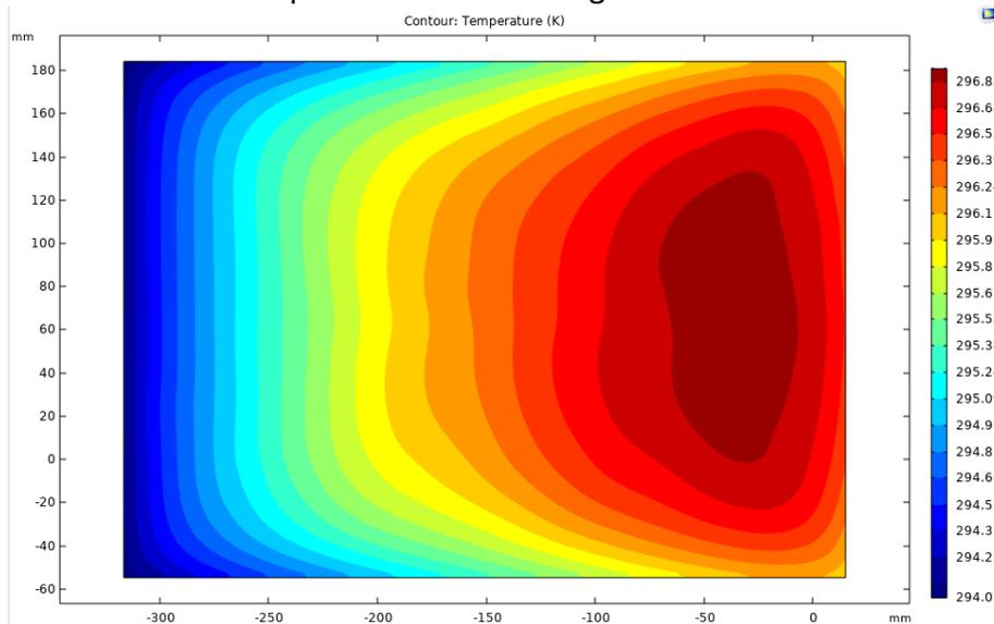
**Fig. 7.** Temperature contour for Expansion-Contraction duct, inlet 145X5 mm
