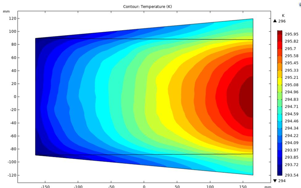
Fig. 13. Temperature contour for a tapered duct with inlet dimensions 175X5 mm
