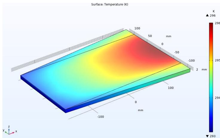
Fig. 12. Tapered duct with inlet dimensions 175X5 mm
