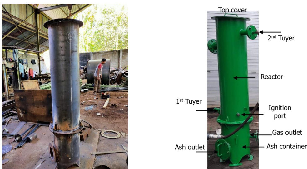
Fig. 1. Photograph of the fabrication process and parts of the gasifier
