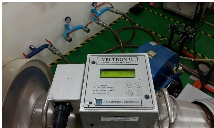
Fig. 4. The Veltron II flow transmitter
