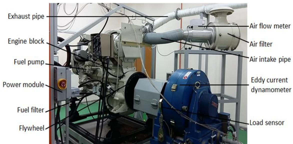
Fig. 2. Full setup of marine diesel engine test-rig
