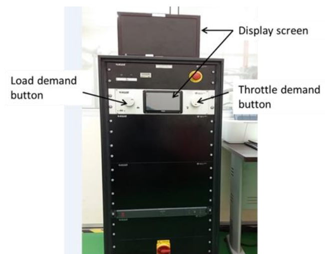
Fig. 5. REO-DCA Data acquisition unit
