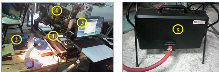
1- Engine, 2- Engine speed control, 3-The computer displays the soot measurement data, 4- NO x measuring equipment (Testo 350 XL), 5- Soot measuring equipment (Msa-pc-se. nr 00601)
