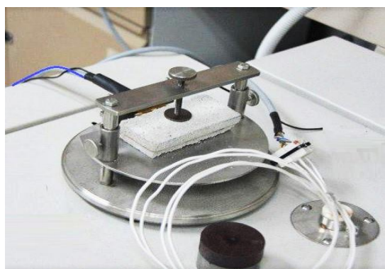
Fig. 2. Set up for the hot disk constant thermal analyser TPS 2500 S
