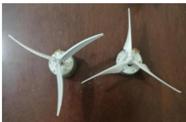
Fig. 16. The two present 3D-printed models; Right: NACA 2412 model, Left: N.Lotus model
