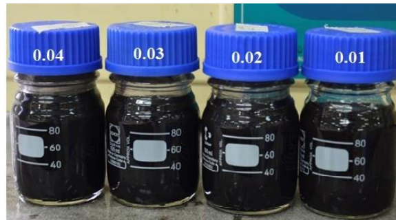
Fig. 6. Samples of CuO/water nanofluids at different volume fractions ( \varphi )
