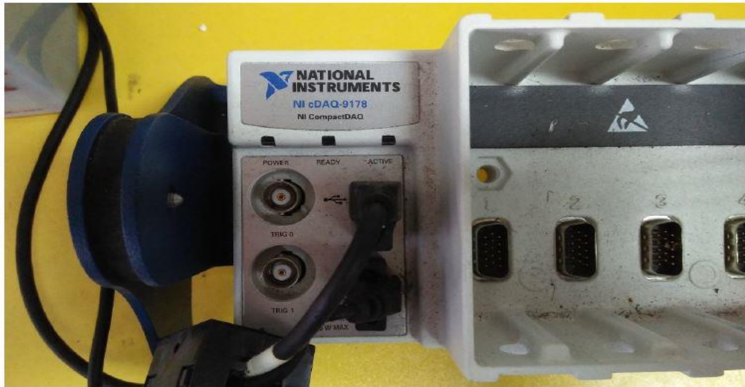
Fig. 3. National Instrument CompactDAQ-9178
