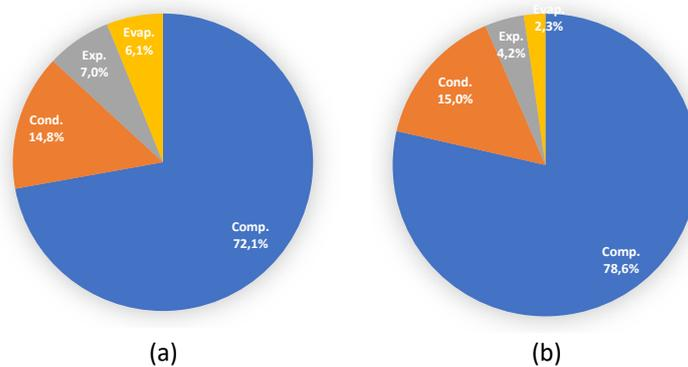
**Fig. 12.** Irreversibility percentage in each component of automotive A/C at 2000 rpm: (a) R134a; (b) R600a
