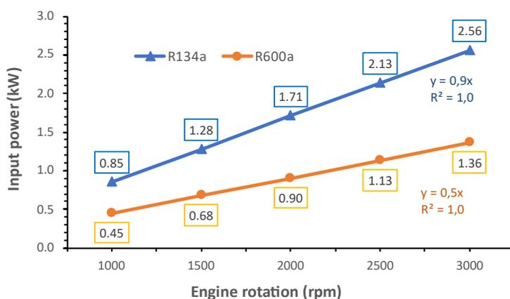
Fig. 3. Input power of automotive A/C for various engine rotations using R134a and R600a
