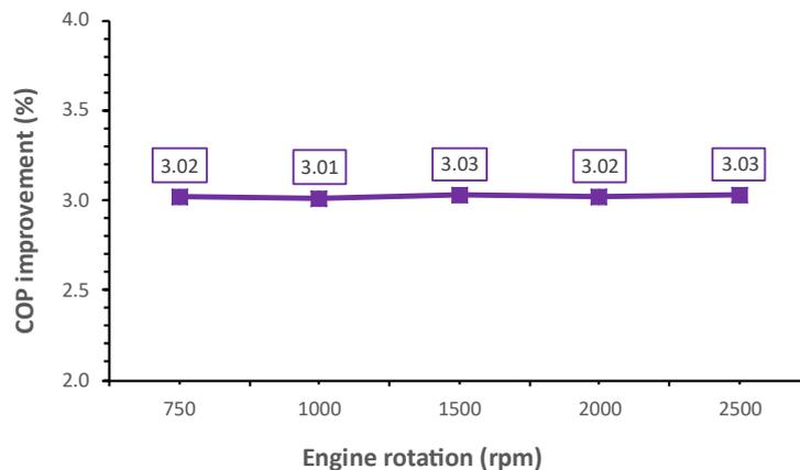
**Fig. 5.** COP improvement of automotive A/C for various engine rotations using R134a and R600a
