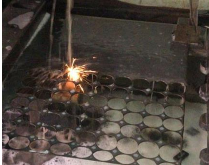
Fig. 1. Sample preparation of HSS substrate by wire-cutting electrical discharge machine
