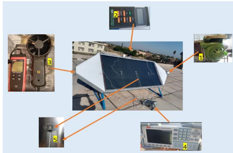
Fig. 2. Experimental work of single pass solar air heater for (1) air blower radial type, (2) solar power meter, (3) airflow meter, (4) the temperature recording data logger, and (5) thermocouples
