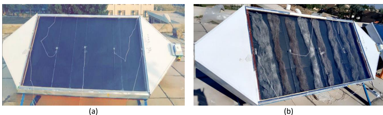
Fig. 1. Displays the experimental set-up for two scenarios of solar air heaters (SAHs): (a) the conventional SAH and (b) the SPSAH with porous media
