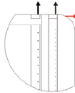
**Fig. 8.** Enlarged figure of orientation for actuator at rear edge of HSB where black and red arrows indicate normal and tangential blowing respectively [17]
