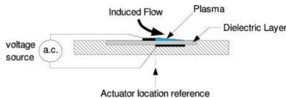
**Fig. 4.** Schematic drawing of SDBD plasma actuator [10]
