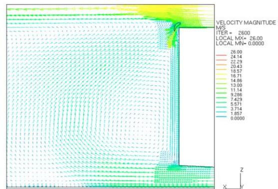
**Fig. 21.** Velocity plot at the back of bus with spoiler installed as viewed from side [39]
