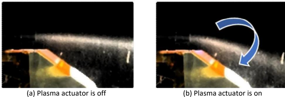
**Fig. 5.** Particle flow visualization at the back of Ahmed model installed with plasma actuator [10]
