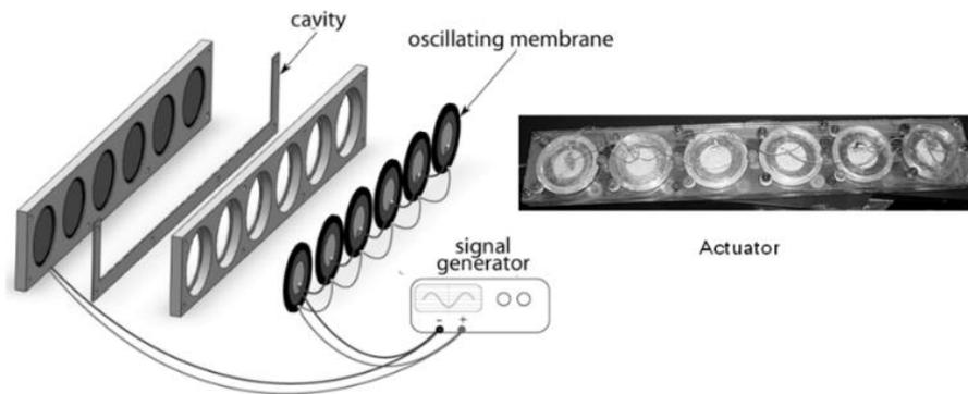
Fig. 13. Piezoelectric actuator used in experiment [30]
