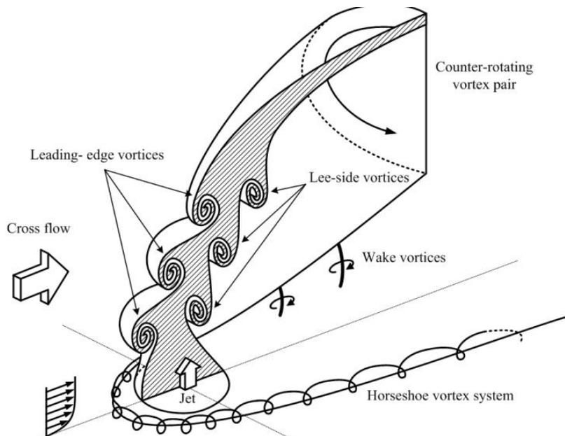
**Fig. 11.** Vortical structure produced by normal blowing jet [19]
