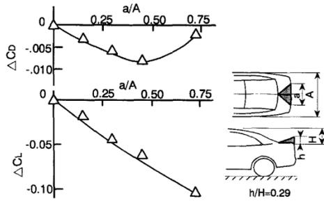
**Fig. 18.** Influence of spoiler dimension on aerodynamic coefficients of sedan car [38]
