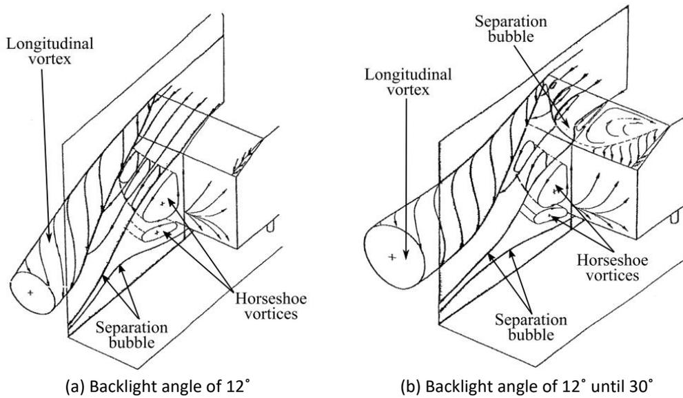
**Fig. 2.** The wake behind vehicle with backlight angle [8]
