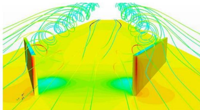
**Fig. 28.** Formation of vortices by rectangular plate VG [59]
