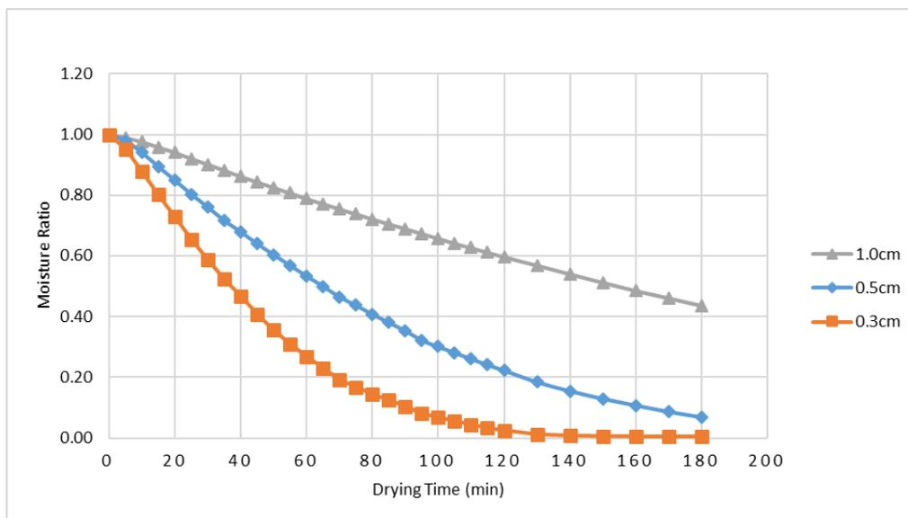
Fig. 8. Moisture Ratio against drying time
