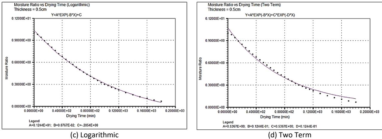
Fig. 11. Comparison between experimental and predicted moisture ratio of 0.5 cm
