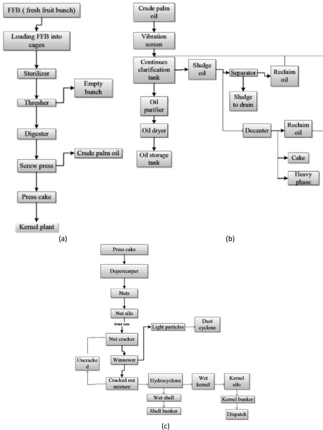
**Fig. 2.** (a) Flow chart of initial extraction process, (b) Flow chart of CPO yield process after screw press, (c) Flow chart of kernel separation process [14]
