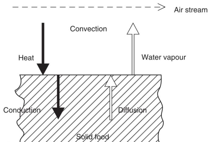
**Fig. 3.** Heat and mass transfer during drying process [18]
