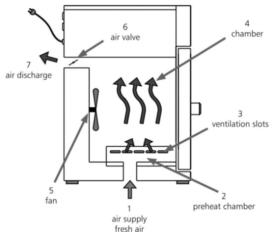
**Fig. 4.** Air flow of Memmert convection oven
