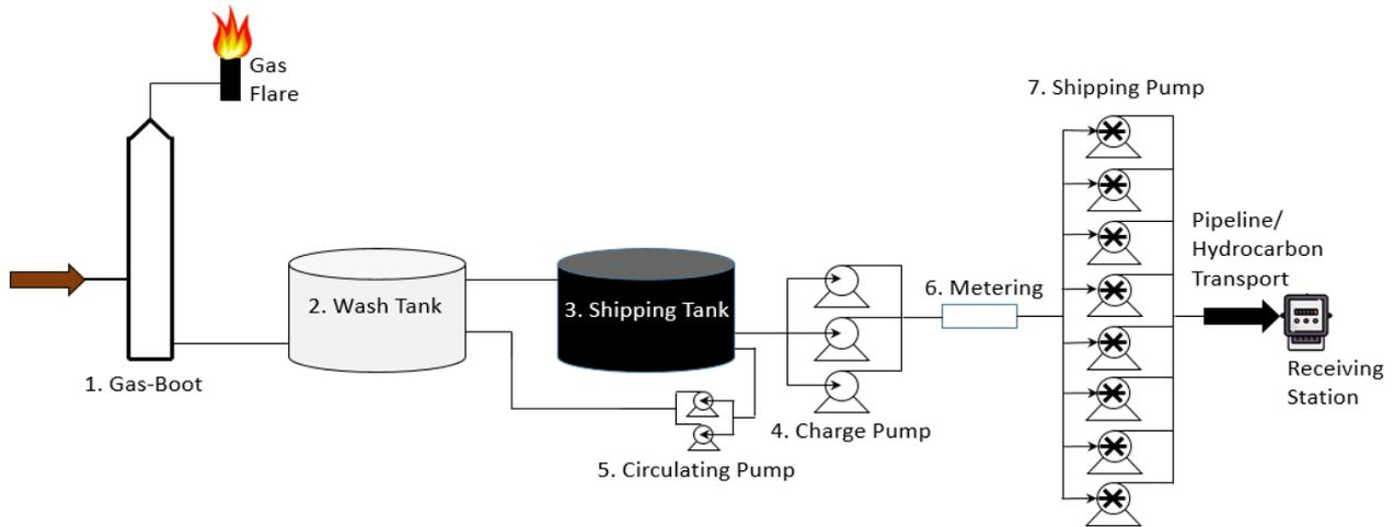
**Fig. 1.** Gathering station and shipping pump process flow
