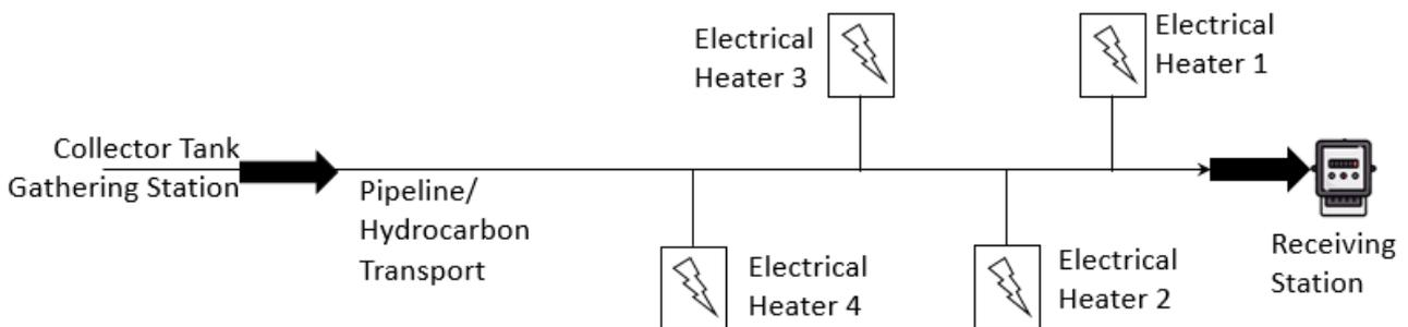
**Fig. 2.** Collector tank gathering station and hydrocarbon process flow
