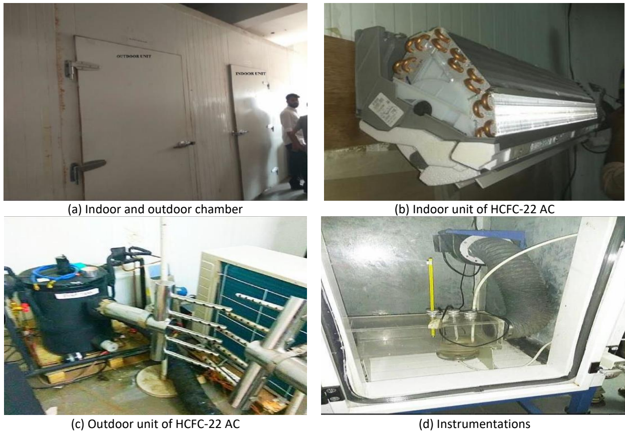
Fig. 2. Experimentation test facility with HCFC-22 SAC unit
