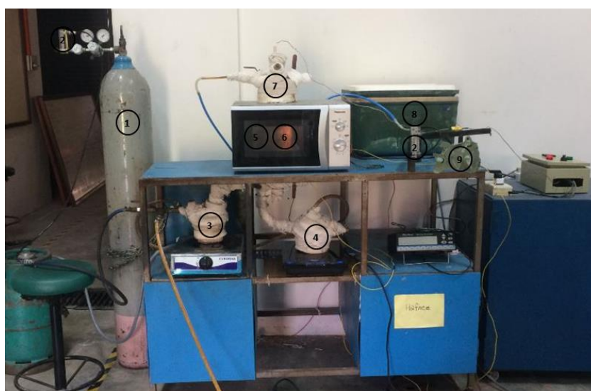
Fig. 1. The photograph of catalytic cracking set up (1. nitrogen gas; 2. flow meter; 3. tar generator; 4. tar tank; 5. microwave reactor; 6. absorber material; 7. asbestos insulation; 8. tar collection; 9. gas bag)
