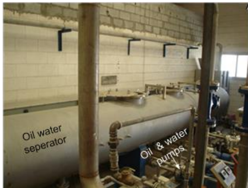
Fig. 1. (a) Multiphase flow loop test facility layout, (b) Pictures oil-water pumps and oil-water flow meters of the multiphase flow facility
