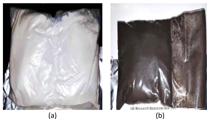
Fig. 6. The photograph of nanopowders (a) \text{Al}_2\text{O}_3 (80 nm) nanopowder, (b) \text{CuO} (80 nm) nanopowder
