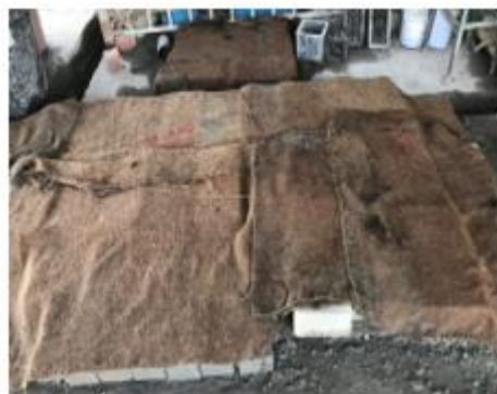
Fig. 3. Wet gunny bag curing for 7 days and 28 days
