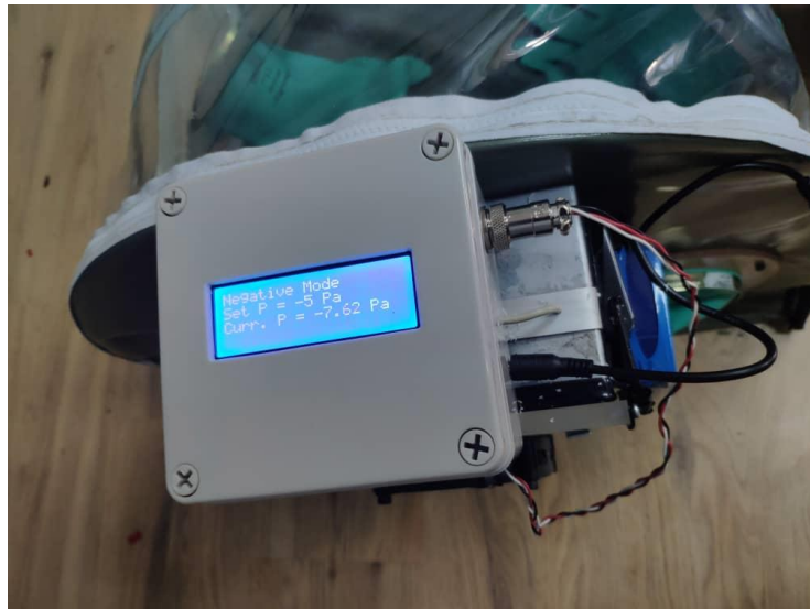
Fig. 4. The blower is stopped when there is vacuum overshoot
