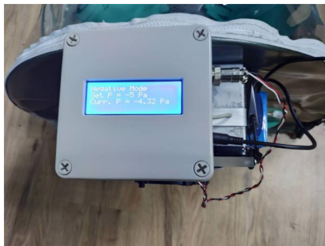
Fig. 3. The blower is running when the desired vacuum is not achieved
