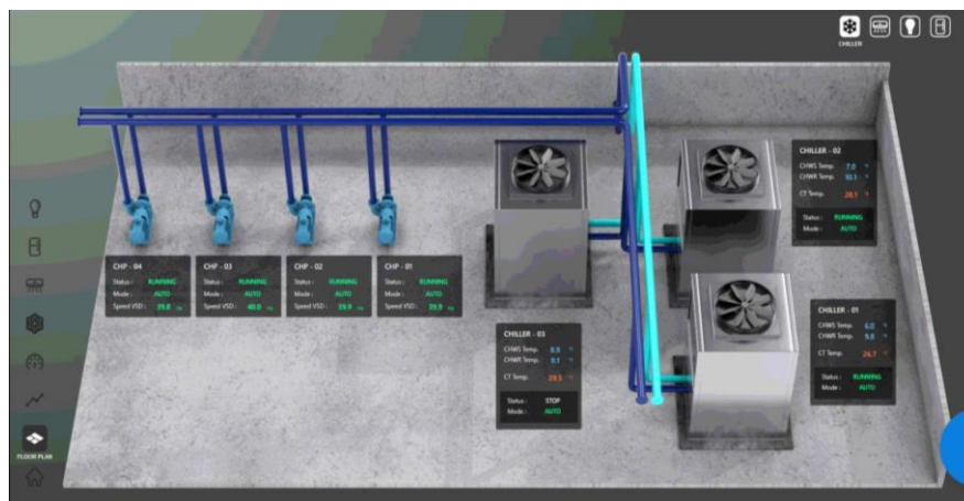
Fig. 9. The REMS for the chiller system
