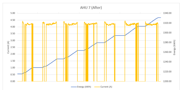
Fig. 25. After Operating Status for AHU No.7
