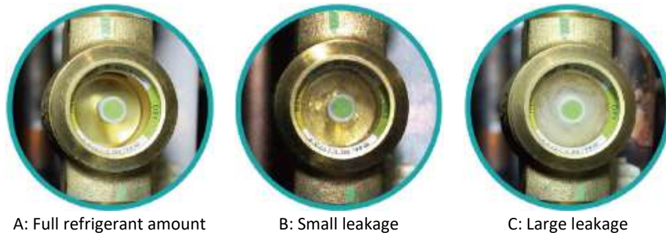
Fig. 3. The appearance of the sight glass in A, B, and C conditions
