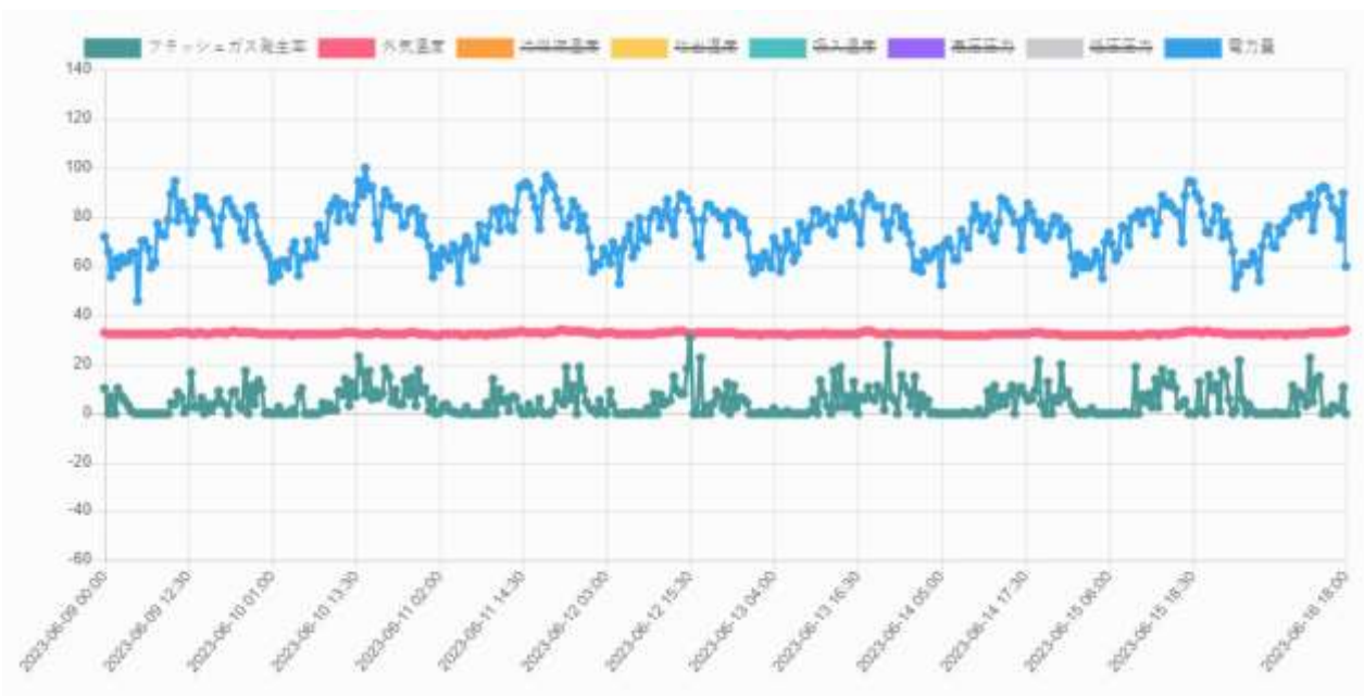
• Flat gas percentage, • Liquid Temperature, • Discharge Temperature Fig. 8. The result of measuring flat gas in 7 Days
