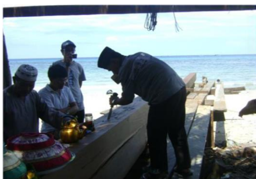
Fig. 2. Positioning and marking of the wooden keel for cutting
