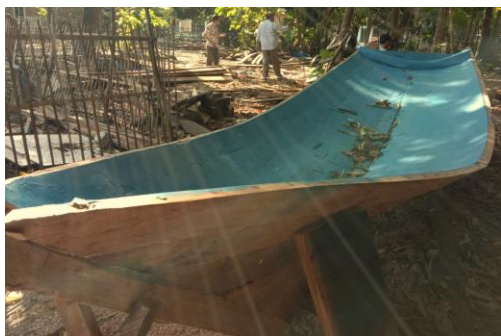
Fig. 5. Part of constructed boat body without frame
