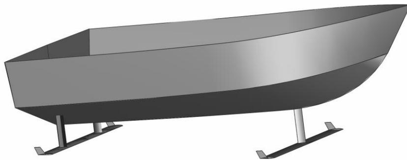
Fig. 1. Hydrofoil craft equipped with winglet
