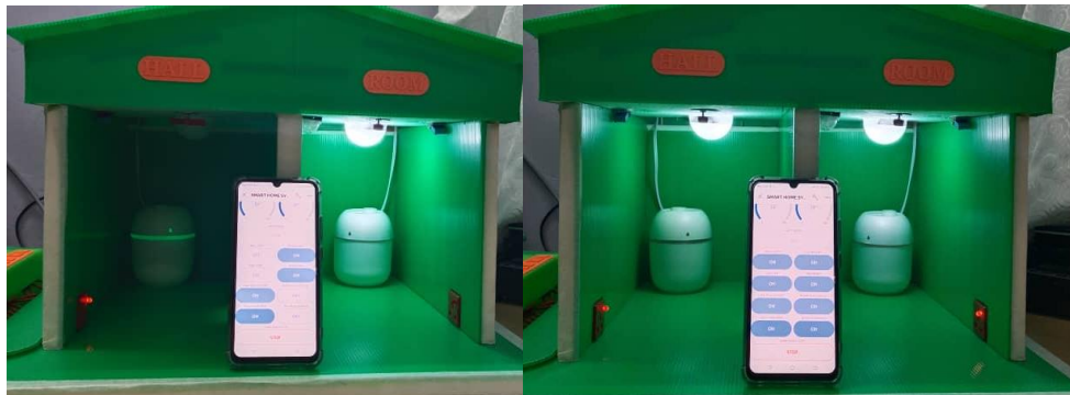
Fig. 9. Hall humidifier, hall plug outlet, room light and room fan are switch on
