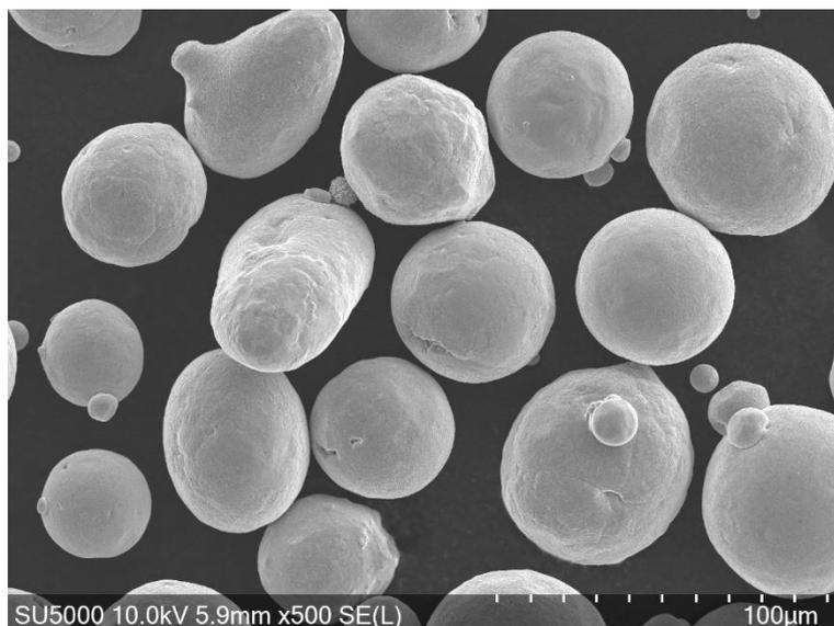
**Fig. 1.** FESEM micrograph of copper particles
