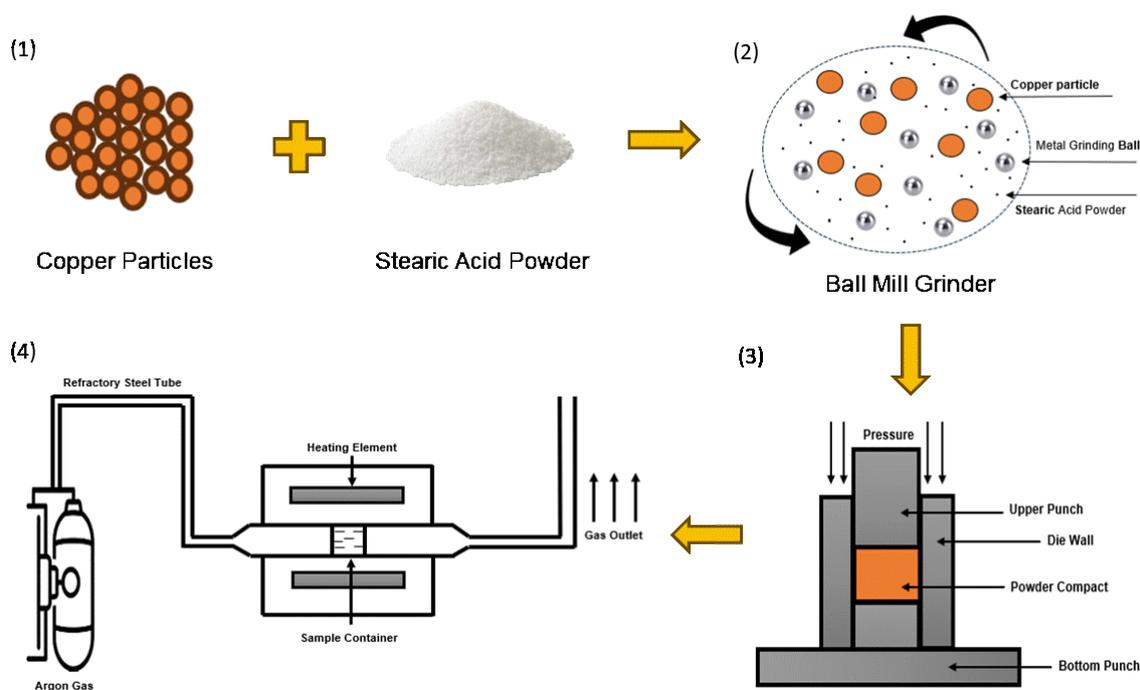
**Fig. 2.** Schematic diagram of copper electrode fabrication by PM process (1) raw materials; (2) mixing; (3) cold-compaction; and (4) sintering operation
