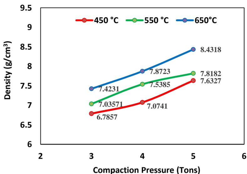
Fig. 3. Effect of compaction pressure and sintering temperatures on the density of PM copper electrode
