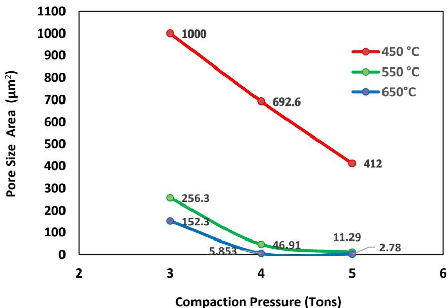
Fig. 5. Effect of compaction pressure and sintering temperatures on the pore size area of PM copper electrodes
