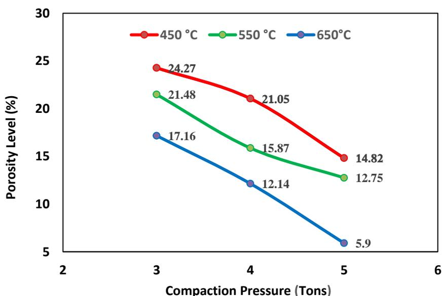
Fig. 4. Effect of compaction pressure and sintering temperatures on the porosity of PM copper electrodes
