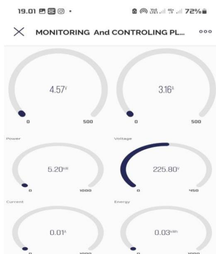
Fig. 6. The monitoring results using IoT of the microhydro power plant in real-time
