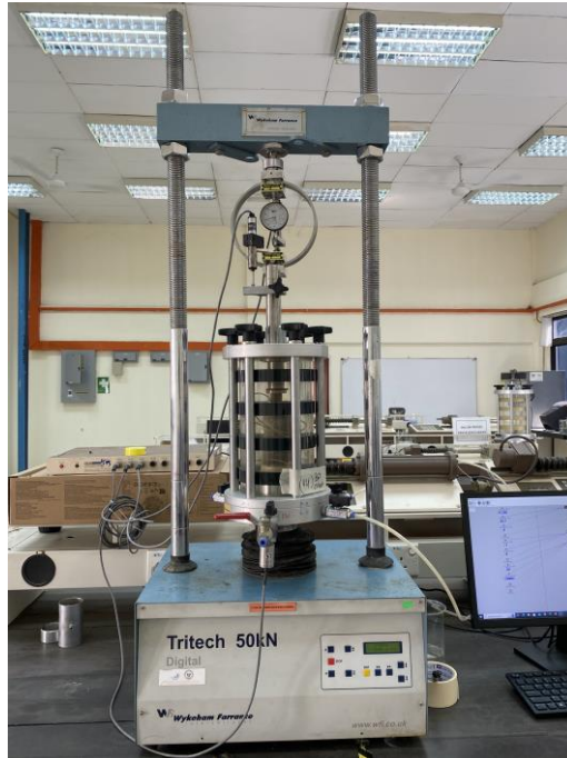
Fig. 1. Triaxial Test – Unconsolidated Undrained set up
