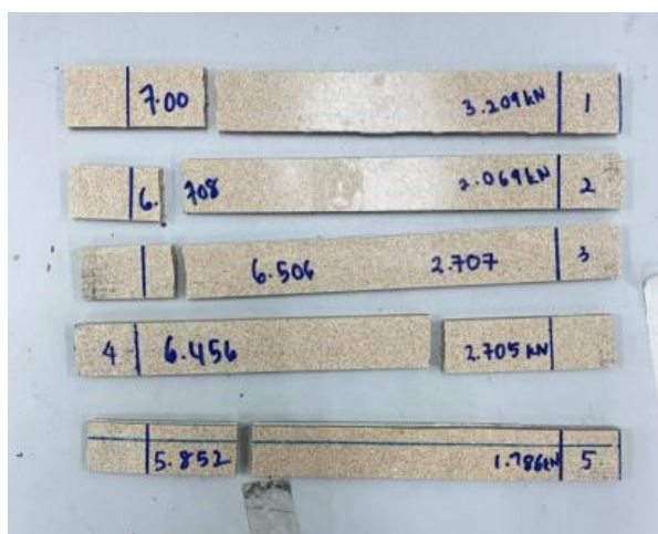
Fig. 4. Specimen of tensile test
