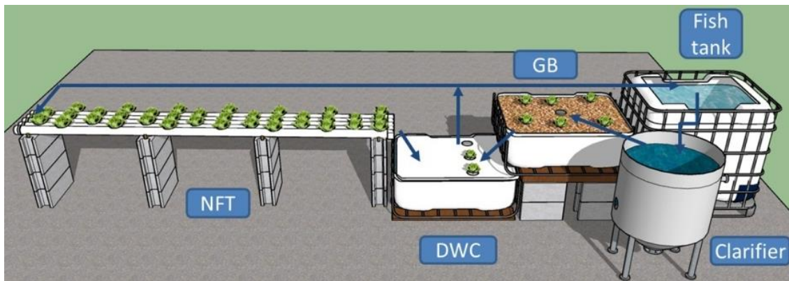
Fig. 2. A 3D model of the micro-scale aquaponic system with the three hydroponic sub-systems
