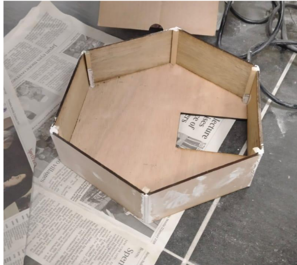
Fig.14. Seat section that is being joined after cutting
