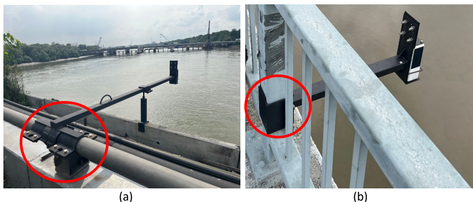
Fig. 3. RMS Camera's structure at (a) Parang Bridge, Klang (b) Kota Bridge, Klang
